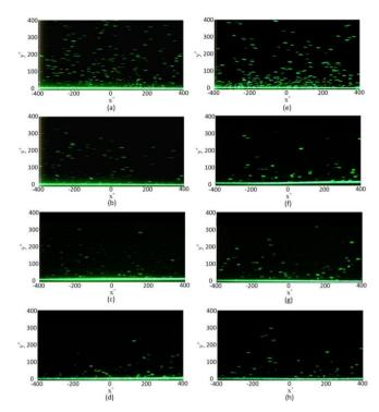
Figure 2 instantaneous distributions of particles in the boundary layer. From the top to the bottom, the rough element size of each row is 0  $\mu$ m, 51 $\mu$ m, 61 $\mu$ m and 120  $\mu$ m, respectively. The left column is for the particles with the Stokes number of 16, the right one for that of 100.
