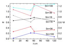
Figure 6 the deposition ratio versus the rough element size and Stokes number, and the ratio of the number of resuspension and that of on the wall
