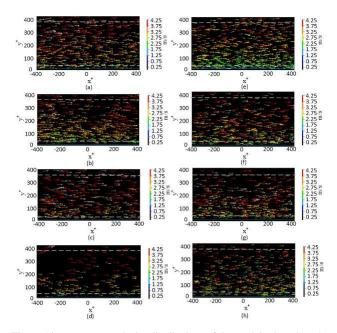
Figure 5 instantaneous velocity distributions of the particles based on the PTV measurements in the boundary layer. From the top to the bottom, the rough element size of each row is 0  $\mu$ m, 51 $\mu$ m, 61 $\mu$ m and 120  $\mu$ m, respectively. The left column is for the particles with Sn = 16, the right one for Sn = 190.
